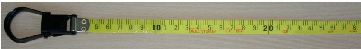
Figure 11: Example of the alternative fibreglass tape with hook end and pull loop (12.7mm width)
