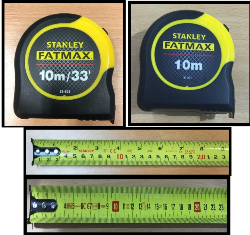
Figure 52 Examples of STANLEY FATMAX TAPE case and blade marking (10m/33ft and 10m)
