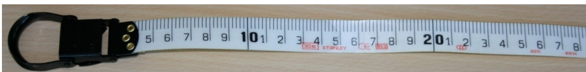
Figure 9: Example of the alternative fiberglass tape with hook end and pull loop (19mm width)
