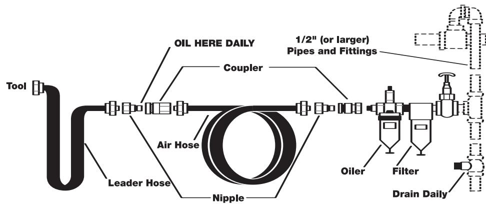
The recommended hook-up is shown in figure A. Pneumatic tools operate on a wide range of air pressures. For maximum efficiency and longer tool life, the pressure of the air supplied to these tools should not exceed the rated PSI at the tool when the tool is running. Using a higher than rated pressure will cause faster wear and drastically shorten the tool's life. A higher air pressure can also cause an unsafe condition.
