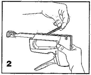
Place stick of staples in bottom channel as shown in Fig. 2 so legs are pointing up.
