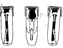
Knob, Lever Cap and Plane Iron Cap removed to show the action of the Lateral Adjusting Lever
