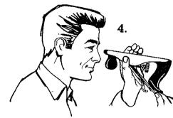
To adjust for the evenness of the shaving sight along the bottom of the Plane and move the Lateral Adjusting Lever toward the right or the left.
