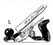
To put the Plane together lay the Plane Iron, bevel side down, on the Frog. Be sure the Roller on the Lateral Adjusting Lever, the end of the "Y" Adjusting Lever and the head of the Plane Iron Cap Screw are correctly seated.
