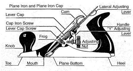
To adjust for the thickness of the shaving sight along the bottom of the Plane and turn the Adjusting Nut until the cutting edge projects about the thickness of a hair.
