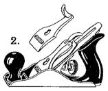
Slip the Lever Cap under the Lever Cap Screw and press down the Cam. If the Plane Iron is in the correct position the Cam will easily snap in place. If the Cam will not snap in place easily, slightly loosen the Lever Cap Screw. If the Plane Iron, is not firmly held when the Cam is in place slightly tighten the Lever Cap Screw.
