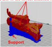
• If the part has a hole or boss that needs to be precisely printed, it is better to place the part standing up so it wouldn't need a support.
