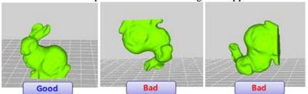
• If the usage of support is necessary, place the model while considering the fact that parts touching the support would be low in printing quality.
