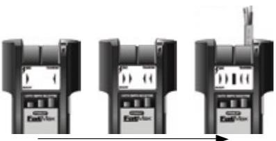
Static electrical charges that can develop on drywall and other surfaces will spread the voltage detection area many inches on each side of the actual electrical wire. To aid in locating the wire position, scan holding the unit  $\frac{1}{2}$ " away from the wall surface or place your other hand on the surface approximately 12" from sensor.
