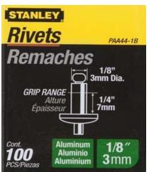
diameter of the rivet which also tells you the size hole you will need to drill or punch. In the example shown to the left, I will need to drill a 1/8 hole for these rivets. The other one listed is called the grip range and this is determined by the total measurement of the pieces of material including any back up plate, or washers you want to bind together with the rivet. This total measurement should not exceed
