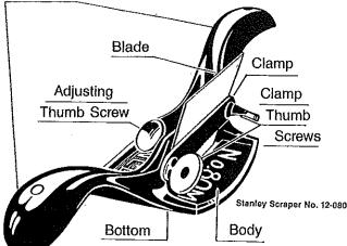
The Cabinet Scraper is used for the final smoothing before sandpapering. It removes the slight ridges left by the plane. It is also used to smooth surfaces that are difficult to plane because of curly or irregular grain.
