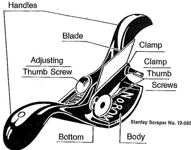
The Cabinet Scraper is used for the final smoothing before sandpapering. It removes the slight ridges left by the plane. It is also used to smooth surfaces that are difficult to plane because of curly or irregular grain.
