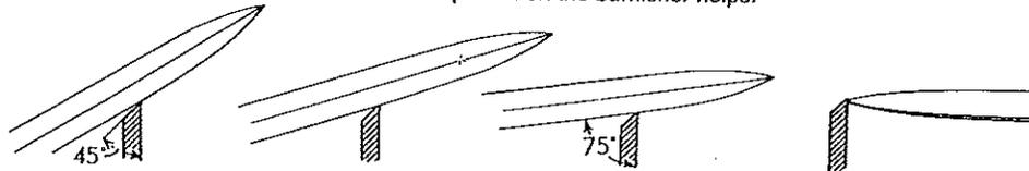
The first stroke should be made with the burnisher held at an angle, a little greater than the bevel. Increase the angle until, at the last stroke, the burnisher is held at about 75° to the flat face of the blade. If the edge should be turned too far over, it can be raised by drawing the point of the burnisher along the edge, under the burr.
