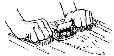
Try the scraper and change the adjustment until it takes a thin even shaving. Hold it turned a little to the side to start a cut. The Cabinet Scraper is usually pushed but it can be pulled. Dust, instead of a shaving, indicates a dull scraper.
