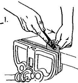
**To Sharpen a Bevel Edge Scraper Blade:**
