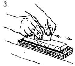
Whet the bevel side of the blade on the oil stone.
