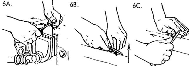
**To Adjust and Use the Cabinet Scraper:** Loosen the adjusting thumb screw and the clamp thumb screws. Insert the blade from the bottom with the bevel side towards the adjusting thumb screw.
