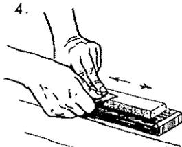
Whet the face side of the blade to remove the wire edge.
