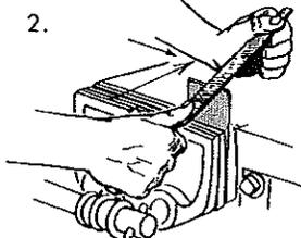
File or grind a bevel of about 45°. Push the file forward and to the side with one sliding motion.
