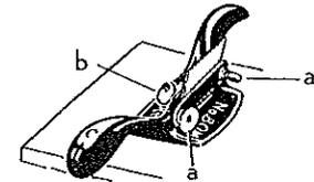
Bring the edge of the blade even with the bottom of the scraper body, by standing it on a flat surface and pressing the blade lightly against the wood. Tighten the clamp thumb screws a. a. Bow the blade by tightening the adjusting thumb screw b, to make it project enough to take a thin shaving. If one corner of the blade projects too far, it can be drawn in by tapping the side of the blade near the top.
