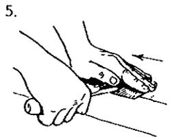
Draw the edge with a few firm strokes on the face side of the blade. Hold the burnisher flat on the face side of the blade.
