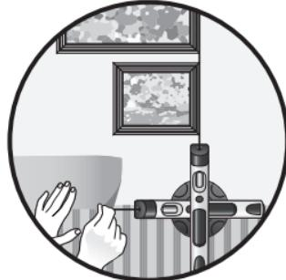
The laser level can be rotated 360° (with 90° references) on the wall/stud mount.
