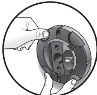
**Use extra caution** when handling the mount. Retractable pins are very sharp. Push the buttons only when you place the mount on the surface of a soft wood or wall-board.
