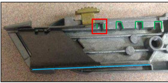
•The bottom of the slider will rest on a platform in the casting (blue line)
