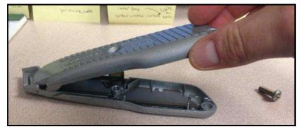
• To close, slide the nose of the left casting on to the right casting at a angle, and the two castings will align themselves.
