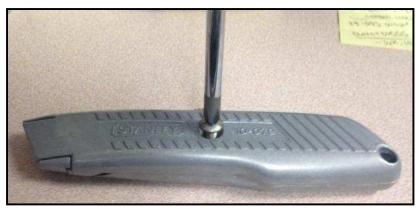
• Tighten the screw to complete the blade change process.
