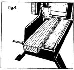
A piece of scrap wood between the clamp and workpiece will eliminate this problem.
