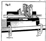
saw to be sure the teeth of the saw are always below the bottom of the plastic
