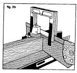
These slides are spring loaded so that they return to their self-storing position upon completion of the cut and removal of the saw. They will also return to their stored position if the saw is just raised in order to place another workpiece in position.
