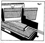
BOARD STOP-refer to figure 3 The adjustable board stop is provided for use when cutting a number of pieces to the same length. It may be attached on either the right or left side of the box, and either on the front or rear of the back plates. If the length to be cut is between the settings obtainable from mounting the stop on the front and rear of the back plate, attach a wooden block to the short leg of the stop and mount the stop on the rear of the back plate.
