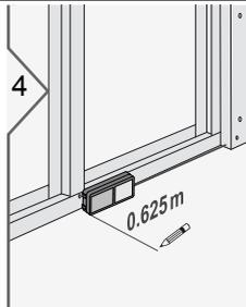
Move device slowly along the stake-out line. The distance to the next stake out point is displayed.
