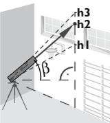
Aim laser at upper points and angle/ height tracking starts automatically.
