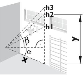
**i** The tracked height "y" is in  $90^\circ$  to the 1st aimed point "x".
