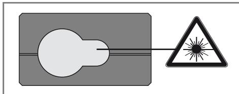
The device produces visible laser beams, which are emitted from the instrument: It is a Class 2 laser product in accordance with:
