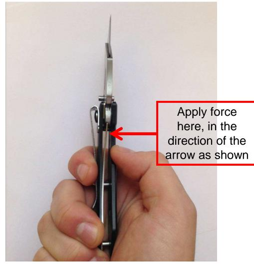
To close a folding knife, you need apply pressure to the liner lock to move it out of the way to allow space for the front half of the knife fold into the handle
