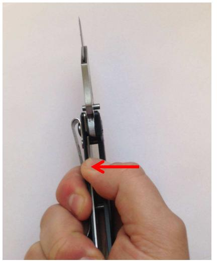
By moving the liner lock out of the middle of the handle, you will now be able to close the knife without interference
