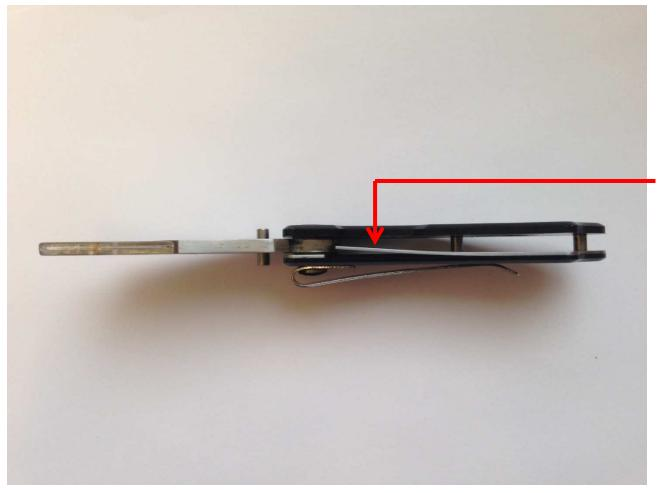
The liner lock extends into the middle of the knife closure area to prevent the front half of the knife from unintentionally closing when in use
