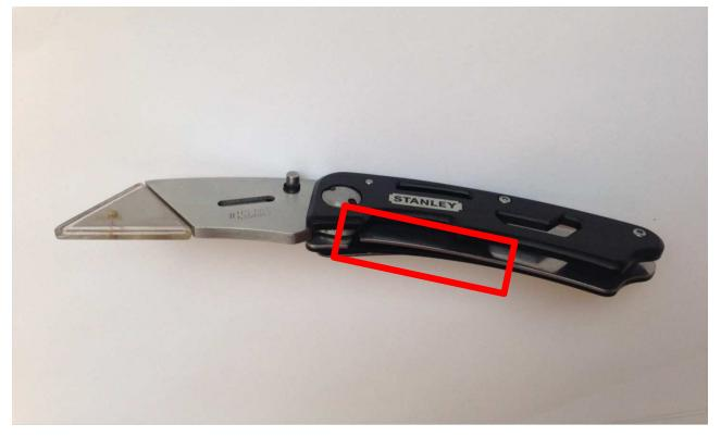
The liner lock is a locking mechanism for opening and closing folding knives
