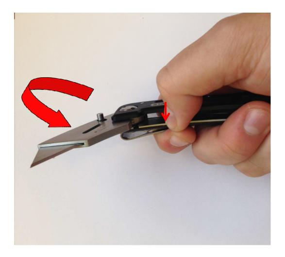
With the liner lock still pressed out of the way, you are now able to start closing the front of the knife into the handle.
