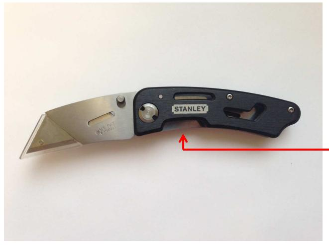
A fully extended folding knife is locked in the open position by a 'liner lock'
