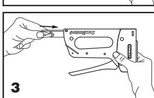
Push slide closed as shown in **Fig. 3**, making sure that latch engages.
