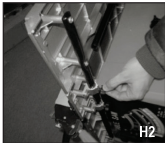
Insert the extension rails into the holes of the table (See Fig. H3)
